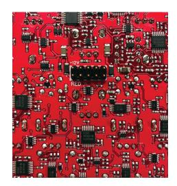
Remove the included power supply cable and take note of the side of the cable with the RED stripe.
