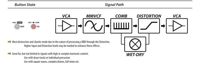
Can be noisy with particular VCF settings and/or less harmonically dense input signals. Use DRY-WET controls and/or DRY-WET and Output VCA CV to dynamically control noise if not desired.
