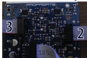
The 3rd PROPAGATE module should have the ribbon cable labeled "2" connected to SLAVE In and ribbon "3" to the MASTER Out header as shown. Connect power normally.
