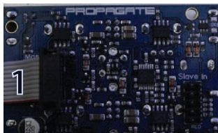
The first PROPAGATE module should have the ribbon cable labeled "1" connected as shown to the MASTER Out header. Connect power as you normally would.
