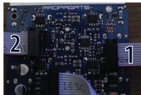
The 2nd PROPAGATE module should have the ribbon cable labeled "1" connected to SLAVE In and ribbon "2" to the MASTER Out header as shown. Connect power normally.
