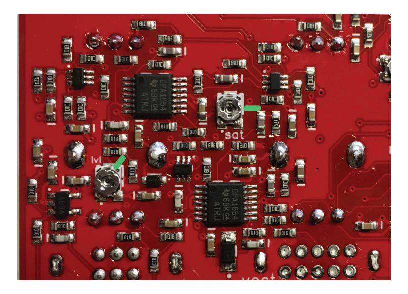
Using the POINTER SIDE, adjust each trimmer to the positions shown by the GREEN lines in the image, above.
