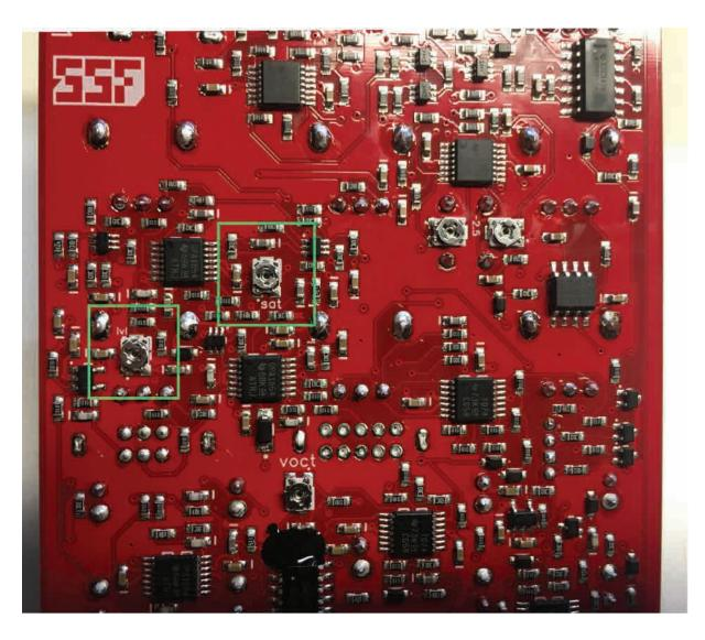
Locate the two trimmers labeled 'lvl' and 'sat', shown above
