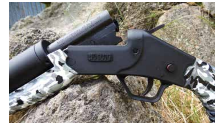
LEFT: The FSS 20g. Note the safety button on the side of the receiver and the forend opening latch above this; both were in a good location and had nice positive actions.
