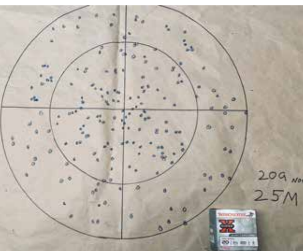
ABOVE: Patterning the .410 model at 20 metres using Winchester Super-X 3\"/>
