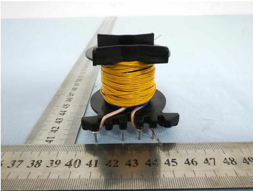
Figure 20. Secondary winding view of transformer
