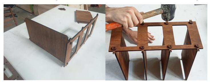
Step 2. Put the other side part and fix all the connections.
