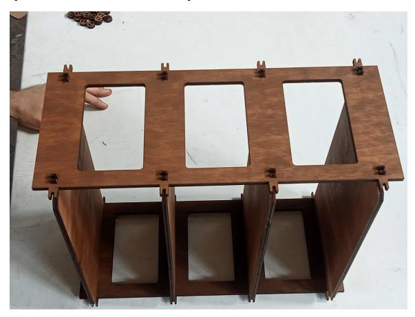
Step 3. Put the front frame on and fix the connections.
