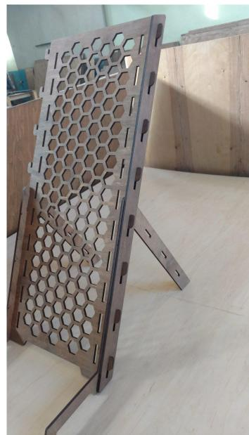
Step 3. Take small "ladder" part, hooks DOWN, put it in the legs grooves and slide it down.
