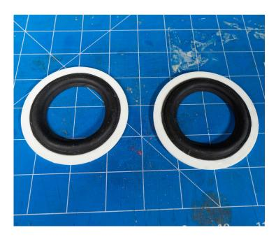
Begin sticking: Carefully attach the surrounds to the lip of the frame sections. Be careful-once the glued sections touch, they bond immediately. Removing them will pull off the glue and require reapplication.
