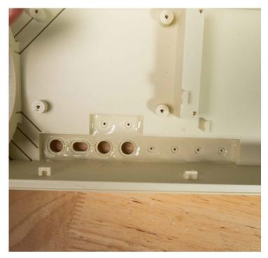
Epoxy Glue Pt 1: Apply a generous amount of epoxy glue to the enclosure where the bracket attaches.
