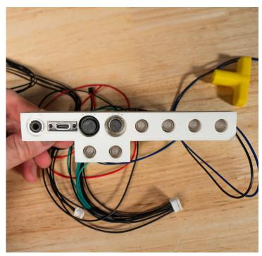
• **Tighten the battery button:** The battery button tightening tool (pictured in yellow) can be used to tighten the nut and securely hold it in place.
