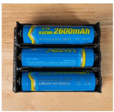
• Batteries: Insert the batteries into the battery board with correct polarity. They may be a tight fit and require some force.
