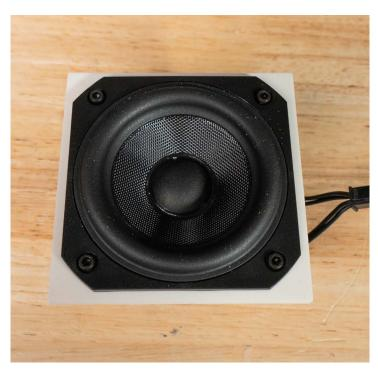
**Screw in the Driver:** Screw the driver in place using the provided screws.
