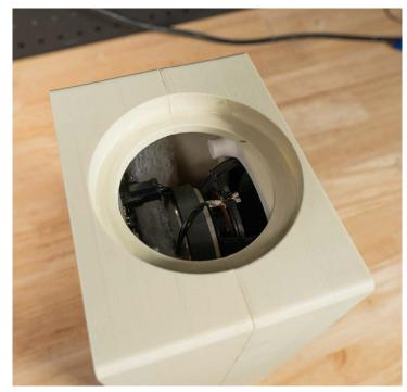
• **Seal it up:** Apply epoxy glue to the mating surface for the passive radiators.
