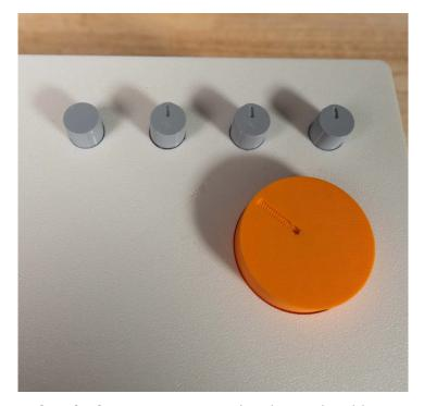
• Glue the button Pt 2: Press the Bluetooth pairing button cap in place and leave to set.
