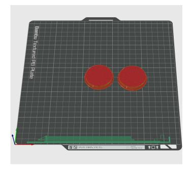
You can print both passive radiator diaphragms at once. The combined weight should be around 27 grams.
