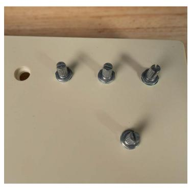
**Nut the Pots:** Firmly attach the nuts over the washers • **Bluetooth Pairing:** Secure the Bluetooth pairing button. to secure the pots in place. It's best to do this before the glue from the previous step cures.
