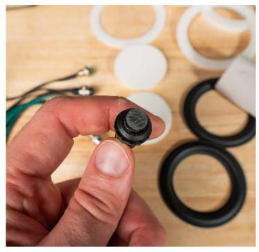
• Rough up the gluing surfaces: Use the provided sandpaper to rough up the surfaces of the power, battery indicator, and Bluetooth pairing buttons. Also rough up the mating surfaces of the passive radiator frames, diaphragms, and rubber surrounds.
