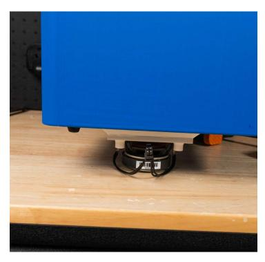
• **Weigh it down:** Using a weight under 5kg, clamp the two parts together while the glue cures. I'm using my trusty Illuminate 5 again.
