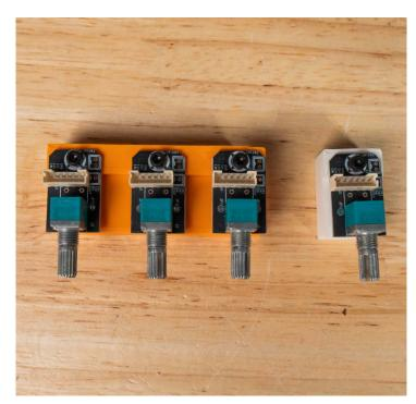
• **Screw the Pots:** Screw the pots firmly onto the pot brackets, ensuring they are aligned straight.
