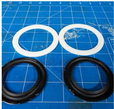
"Contact Glue: To assemble the passive radiators, we'll use the provided E6000 glue. This is a contact adhesive, which means it's applied to both mating surfaces and allowed to dry for 5-10 minutes before pressing them together.
