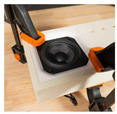
**Mount the Driver:** Using epoxy glue, glue the assembled driver and recess into the enclosure. Use clamps to hold it in place while it cures.
