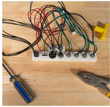
Power Button Wiring: Take the unterminated 2-pin cable from the 'Functional Cables Kit for JAB3+,' cut it to 15cm length, and solder the wires to the power button.
