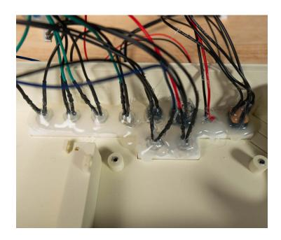
• Hot Glue: Once you're satisfied with the position and color of all LEDs, cover the back of the bracket with hot glue. Ensure you cover the back of every button, LED, and port. This is critical to prevent air leaks.
