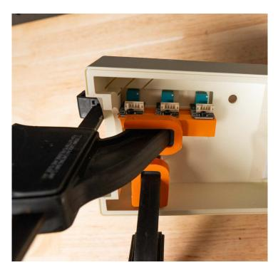
• **Glue the Pots:** Apply epoxy glue to the mating surface of the brackets and attach them to the enclosure with the pots extending through the holes.
