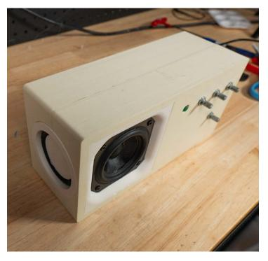
• **The Final Test:** Press fit (dont glue) the passive radiators and conduct a final test to ensure there are no leaks or rattles and everything works.
