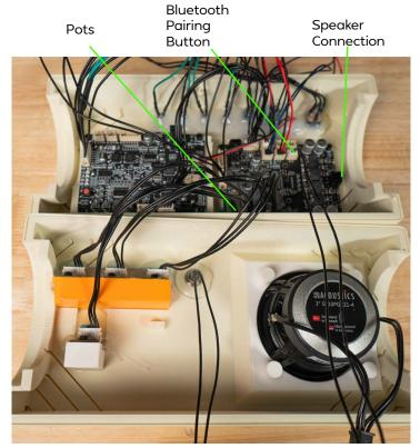
• Connect it all up: Connect all the wires from the front enclosure half. The pots are labeled on the board.
