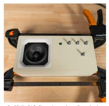
• **Seal it Up Pt 2:** Clamp the passive radiators in place, applying pressure to the frame, not the diaphragm.
