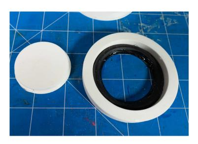
• **Glue the Diaphragm:** Apply E6000 to the lip of the diaphragm and the inner lip of the surround.
