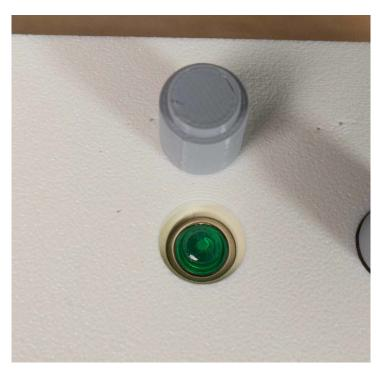
• **Glue the button:** Apply a small drop of epoxy glue to the Bluetooth pairing button. Too much glue will ooze out and jam the button.
