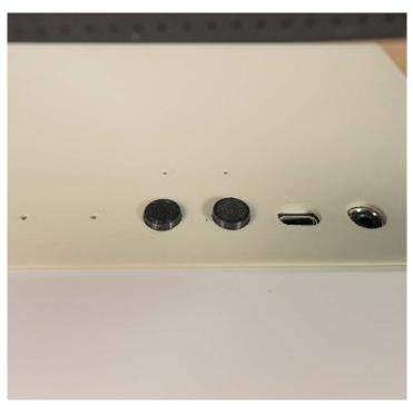
**Glue the Buttons:** Apply a small drop of epoxy glue to • **Glue the Buttons Pt 2:** Press the button caps in place
