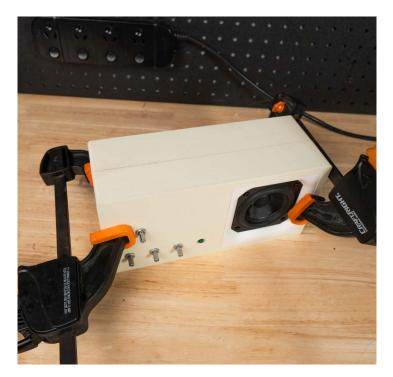
Clamp the Halves: Clamp the two enclosure halves together.
