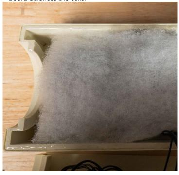
• **Glue the halves:** Apply a generous amount of epoxy glue to one enclosure half. Keep the glue out of the groove—it's designed to prevent excess glue from oozing out.
