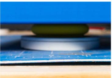
Stick the Diaphragm: Using the diaphragm sticking tool, press the surround onto the diaphragm. Place weight on top to apply pressure while it cures for at least two hours. Having two tools allows you to work on both diaphragms simultaneously.
