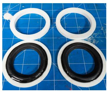
• **Glue the frames:** Apply E6000 to the mating surfaces of both frame sections and the previously assembled surround-frame unit. Allow to sit for 5-10 minutes.
