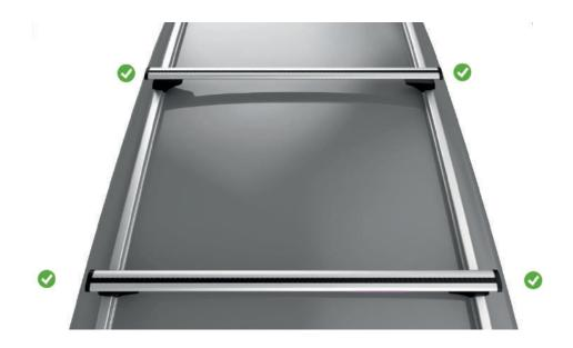
To check the fitment, firmly grasp load bars and attempt to move forward and backwards, side to side.
