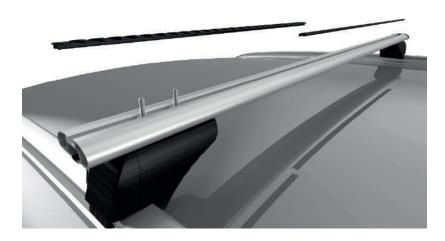
Take the rubbers off and insert T-Bolts. Insert the rubbers again after you remove T-Bolts.
