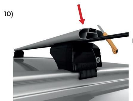
Remove the upper cover, insert the rubber to the below, cut the extra.
