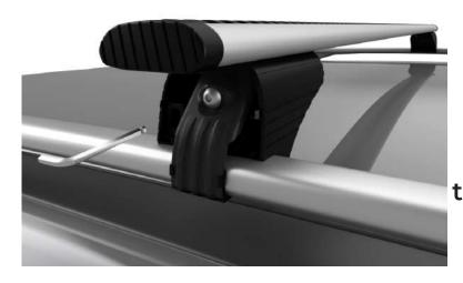
Go back to the first side and tighten it fully. Then, move to the other side one more time and fully tighten that one, too.
