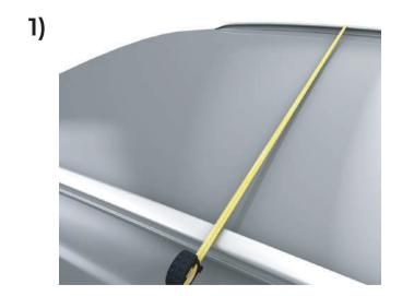
First, measure the area between your roof rails on rear side.
