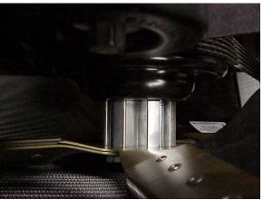
will cause dangerous wobble in the fan blade. This thing holds the fan spinning at several thousand RPM's and has to be precision or damage may result to you or your vehicle. Mount the fan and spacer with the shipped Hayden bolts. These will work fine in the length provided.
