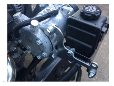
The 5/8" 90 degree hose barb we install in our pumps can be re-clocked or rotated to adjust the angle to match your return hose. Place a wrench over the flats on the barb and turn. The barb is installed with a slight press fit and has non-hardening sealer which will not be damaged by re-adjustment.
