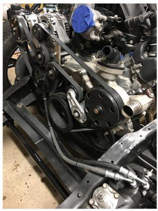
Gear Box Hoses: Pressure hose port on left in photo, return hose port on right
