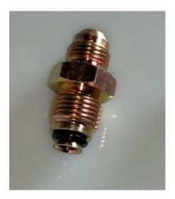
Install a straight conversion fitting in the power steering pump.
