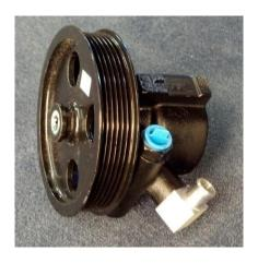
Above: Typical PS pump with 6-groove pulley and custom 90 degree hose barb installed
