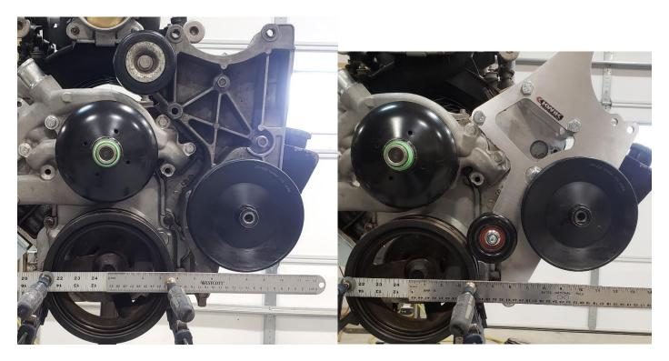
Above left: OEM truck alt/ps bracket with P series pump. Bottom of pulley is slightly above center of crank. Outer edge of pulley is approximately 11.25" from center.
