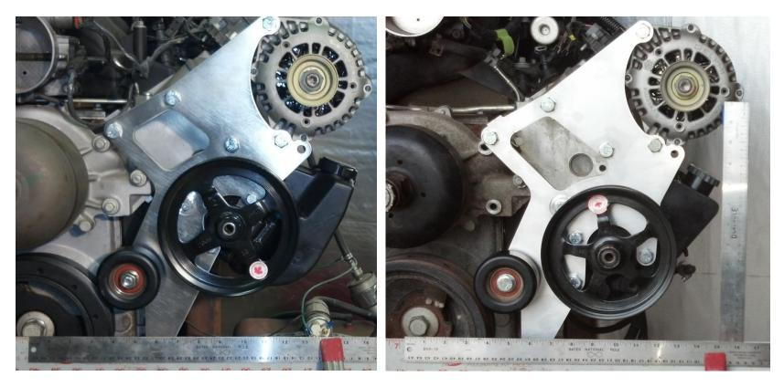
Note the center lines of the Type II with attached reservoir (left) compared to the P Series pump (right). Both have an overall width of about 15" but the P Series pulley is lower by about 1.25"
