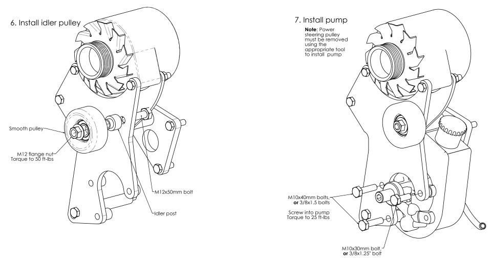
Screws into pump Torque to 25 ft-lbs
