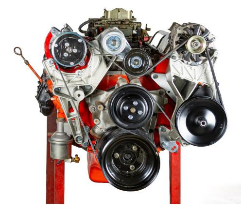
Step 9. Install belt. Suggested belt is Gates K060955. Verify tensioner is in the middle of its travel both after installation AND after initial startup. Longer or shorter belt may be required.
