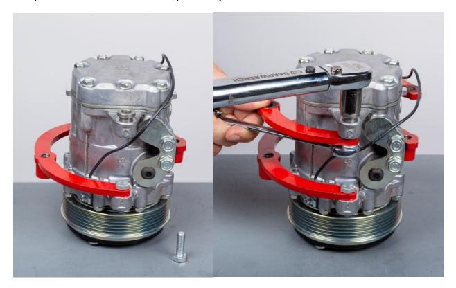
Step 1. Make sure rear sleave of compressor is pushed out so that it is flush in the inside as shown.
