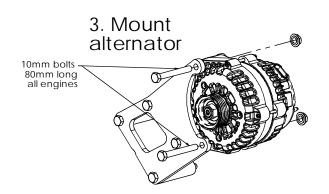
4. Torque all 10mm fasteners to 37 ft-lbs.
