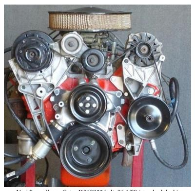
No idler pulley – Gates K060955 belt, 96 1/8" (standard deck)
