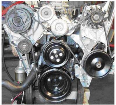
With idler pulley – Gates K060966 belt, 97 1/8" (standard deck)
