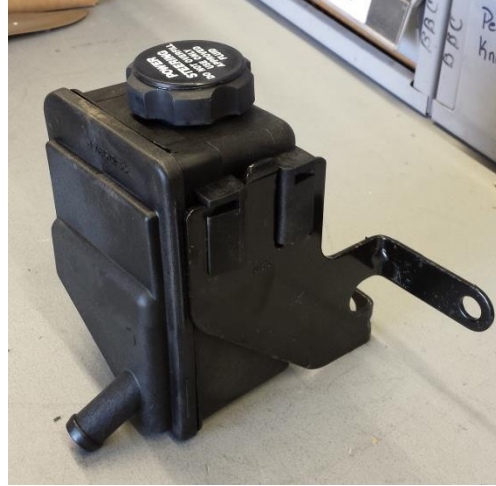
Left above: Conventional reservoir front mount. Right above: Spring mounting clip can be reversed for mounting on firewall, inner fender, core support, etc.
