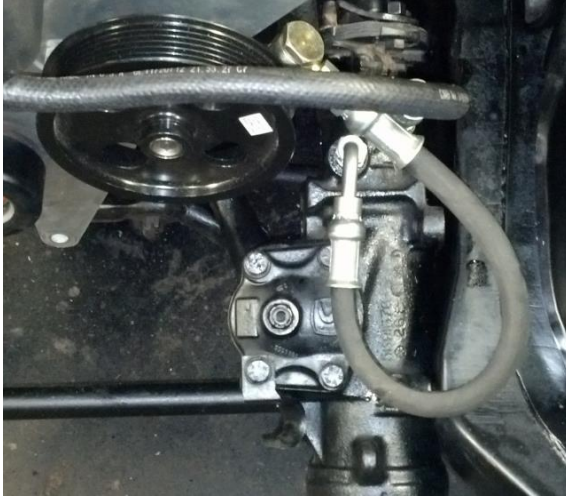
Gear Box Hoses: Pressure hose port on left in photos, return hose port on right
