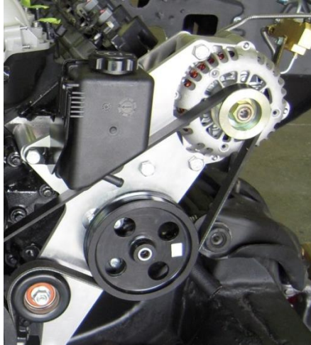
Left above: Conventional reservoir front mount. Right above: Spring mounting clip can be reversed for mounting on firewall, inner fender, core support, etc.
