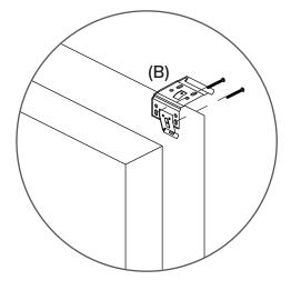
(B) Outside Mount - Mount the brackets on the surface of wall or window frame.
