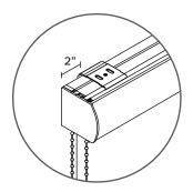
Brackets must be installed no more than 2" from each end of the cassette. A third bracket will be provided for shades wider than 72" and can be installed halfway between the two outer brackets.
