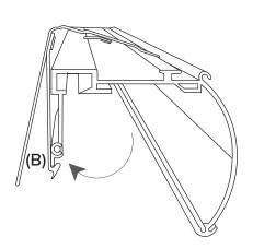
Attach the cassette to the mounting brackets by (A) hooking it under the front lip of the bracket and (B) push the bottom front of the headrail backwards into the rear lip of bracket, CLICK it into place at the rear.
