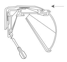
Insert a flat head scewdriver between the cassette and bracket as shown. Pry gently on the spring clip to unlock it from the bracket. The cassette should then disengage from the bracket. EASY BLINDS ZEBRA SHADES Page 4 of 4
