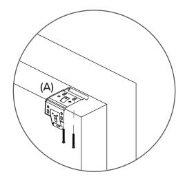
(A) Inside mount - the brackets within the window frame.
