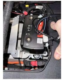
STEP 2: Remove Factory M4 Screws on your CTEK Smart Pass. Using X4 of the replacement Longer M4 screws provided, Take your GP Mounting Bracket and sandwhich under the CTEK Smart pass and the factory Mounting bracket of the Smart pass. Notice the orientation. The GP logo goes under the Smartpass. Use M4 Screws to remount the Factory CTEK Smartpass.
