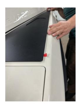
STEP 5: 3M VHB needs at least 12-24 hours to bond properly for the adhesion to work. Please avoid driving for 24 hours or exposing the fender plate to the elements. Please reference the 3M VHB Technical Data sheet for more information. Full Bond is in 72 hours if installed correctly.
