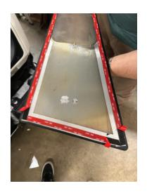
STEP 3: Place your Fender plate on the clean surface of your fender, insuring it is lined up in the position that you want it with the red film tabs exposed. DO NOT press down heavily on the plate as you are lining it up and using the exposed tape sections to hold it in place.
