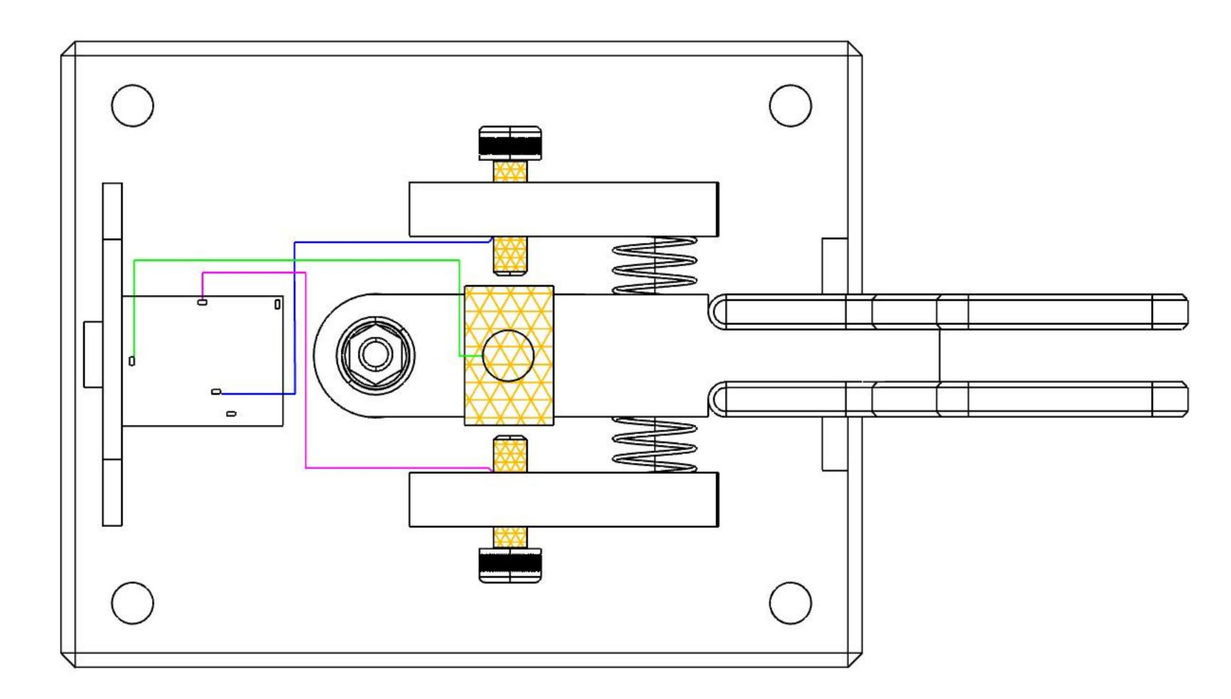
lambic Morse Code Single Arm Paddle 2 Double Sealed Ball Bearings Stainless Steel Hardware Solid Brass Contacts Adjustable Gap Sets Made In the USA
