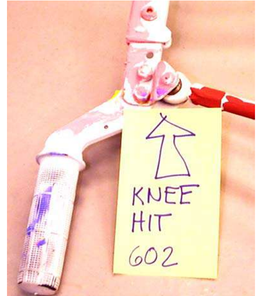
Figure 6. Edge of nut that caused knee cut on the underside of the hand control.
