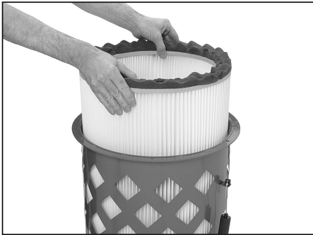
Figure 65. Removing the filter from the canister assembly.
