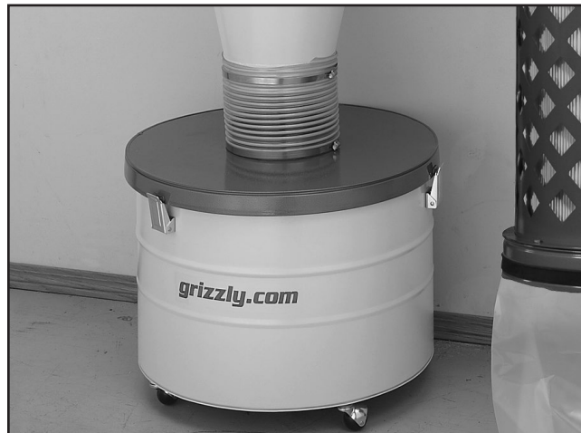
Figure 30. Drum attached to cyclone funnel with clear 9" hose.
