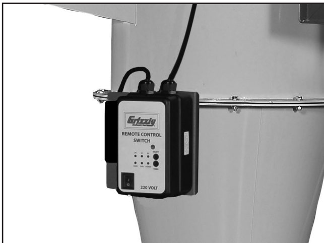
Figure 33. Switch mounted to funnel.
