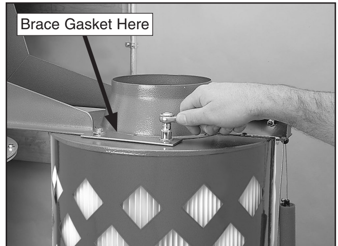
Figure 19. Mounting filters to the braces.
