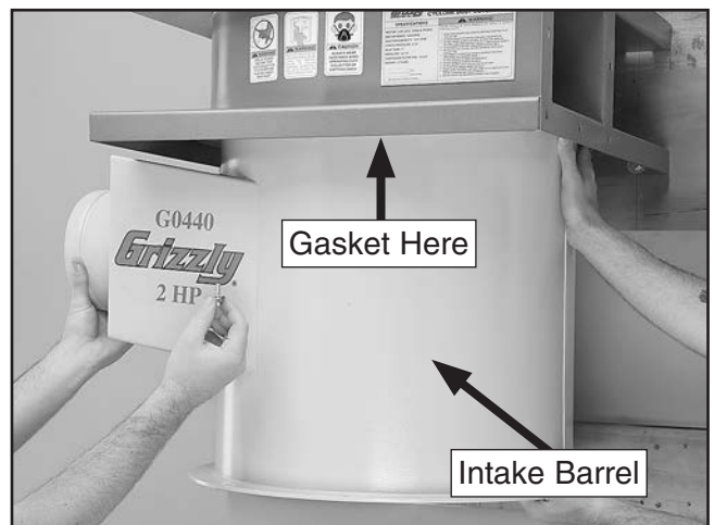
Figure 9. Securing blower on intake barrel.
