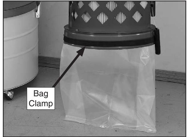
Figure 28. Plastic collection bag clamped in place under filter.
