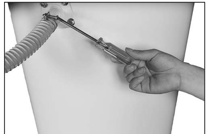
Figure 13. Cyclone vacuum tube and hose attachment.
