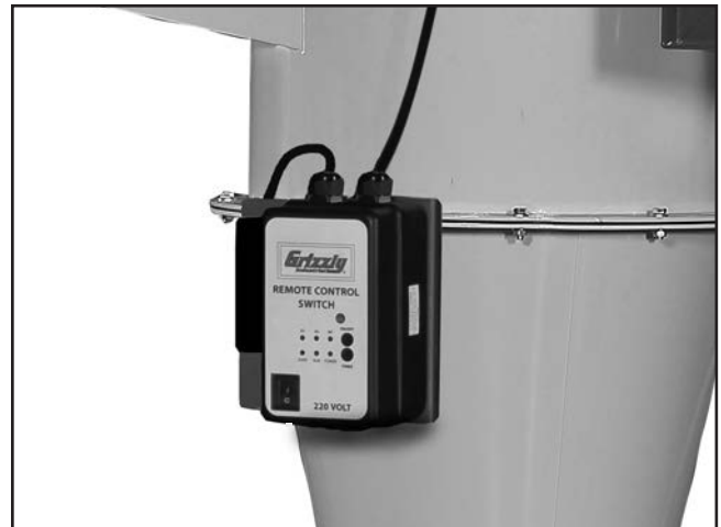
Figure 29. Switch mounted to funnel.
