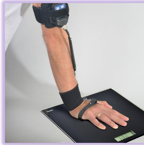
Figure 4-7 Using bathroom scale as reference level for contact force calibration
