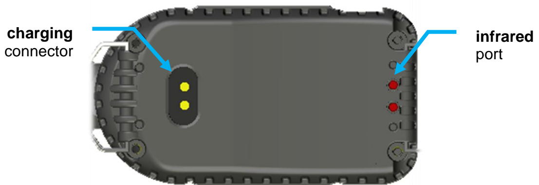
Figure 3-3 SV 103 back view - charging and infrared port (reserved for future use)
