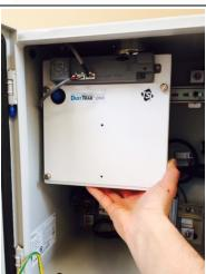
Attach RH/Temp Sensor cable to heated inlet control module.
