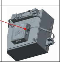
17. If using a Thiamis 1000 Node, route the other side of the cable to the power input on the Thiamis node.
