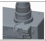
14. Attach ferrite to cable with one wrap of the cable and snap the ferrite together (enclosure not shown for clarity).
