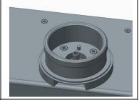
Push out elastic plug and install RH/Temp Sensor Gland to side of environmental enclosure.
