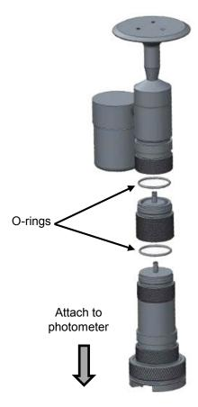
8. Attach column to Photometer inside Enclosure.
