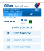
15. The Home Screen allows you to perform remote monitoring of the connected GilAir Plus pump.
