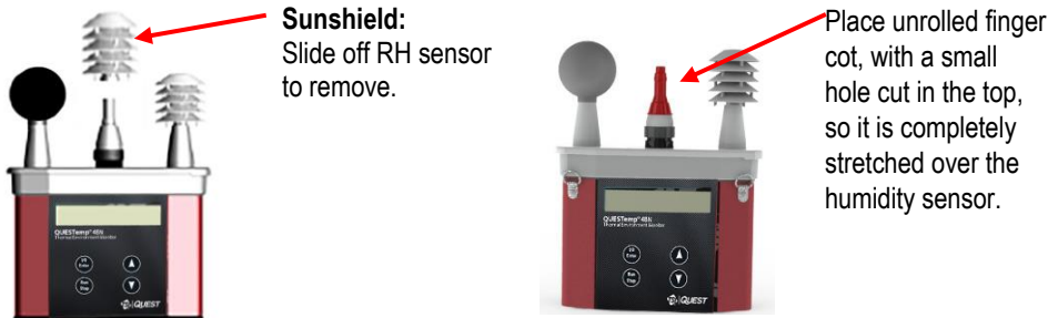
Figure 1-26: Sunshield & placement of finger cot prior to RH alignment
