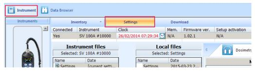
5) Download current Settings from Instrument files to Local Files using right arrow and edit SV103 settings using panels on the right hand side
