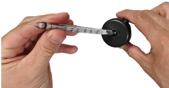
Figure 8: Breaking off both tips of a detector tube
