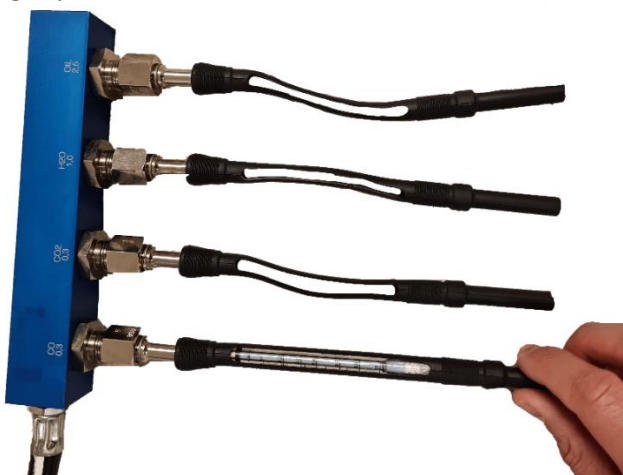
Figure 9: Placing the detector tube in the rubber tube holder
