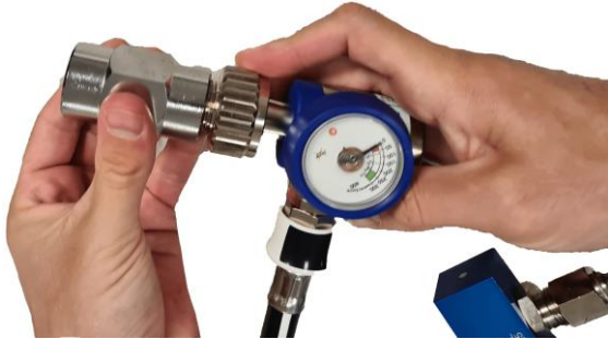
Figure 3: Screwing the adapter on the pressure reducer.
