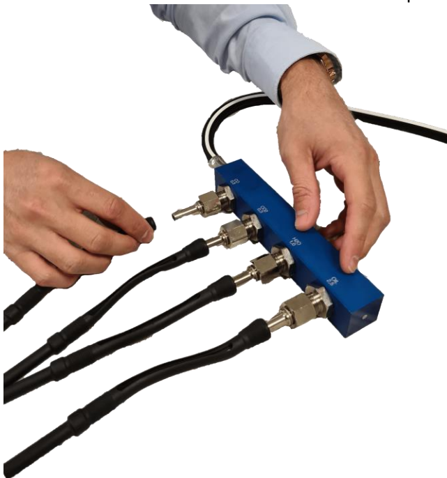
Figure 7: Connecting rubber tube holders to the manifold
