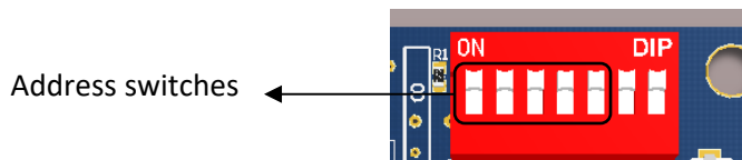
Diagram 9: BTN Series detector address switches
