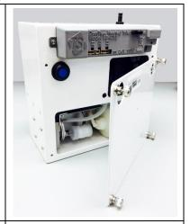
Remove the four (4) Phillips-head screws from the left side panel.
