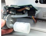
Place new pump into photometer case with muffler orientated at the bottom.
