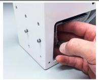
8. Replace photometer service panel and reinstall photometer inside environmental enclosure.
