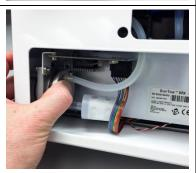
Secure pump module in instrument case with four (4) Phillips-head screws on left side.
