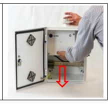
Disconnect the vacuum tube, muffler, and power cable from pump module.
