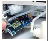
5. Obtain replacement pump. Connect muffler to (P), vacuum tube to (V), and power cable.
