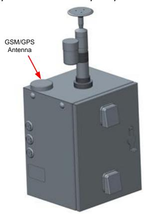
3. Run GSM/GPS antenna cables through the antenna post and screw the antenna to the antenna post. Attach the antenna post and antenna to the enclosure as show if you purchased a solar shield.
