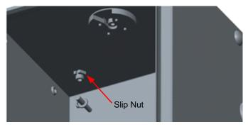
5. Using 7/64" Allen wrench and socket head screws attach adapter plate to DustTrak. Using 1/8" Allen wrench and button head screws attach the Thiamis unit to the adapter plate.
