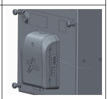
7. Connect power connector to DIN Rail.
