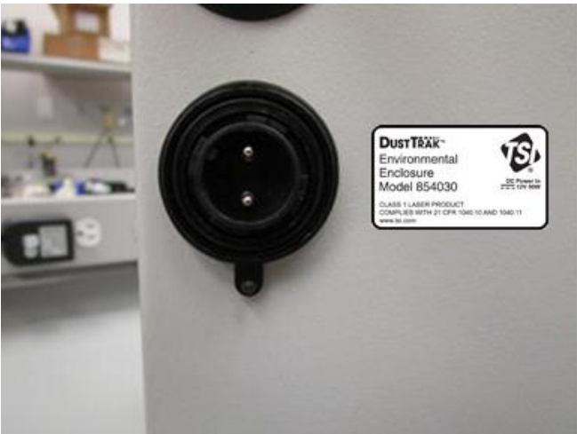
Figure 20:DC Power Label
