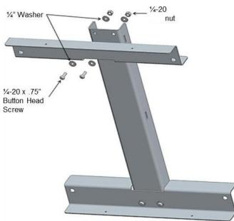
Attach the pole mount to 4 locations on the environmental enclosure using the provided 3/8" screws, washers, and nuts.
