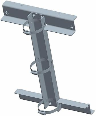
4. Position the enclosure and attached pole mount against pole at the desired height and tighten hose clamps using a 5/16" nut driver.
