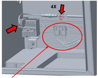
Battery connection harness shown where connection to batteries will be made in next step below.
