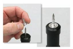
**Step 1:** Load a sample probe onto the piercing tool.
