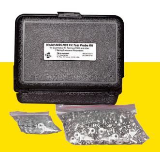
The kit includes 500 lightweight disposable sampling probes and easy to use installation tools. It only takes a few seconds to puncture the mask, insert a probe and then press a push nut on from the other side. The PortaCount Pro+ Fit Tester sample hose fits directly onto the exposed end of the sampling probe.
