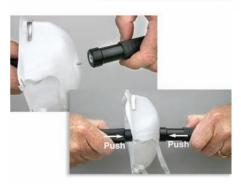
**Step 4:** On the outside of the respirator, align the push nut tool over the end of the exposed point. Hold the tools in-line with each other and firmly push them together as far as possible.
