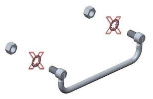
3. Position the 3/8" washers on the exterior of the enclosure. Install the sealing washers on the interior with the rubber side of the sealing washer facing the enclosure surface.
