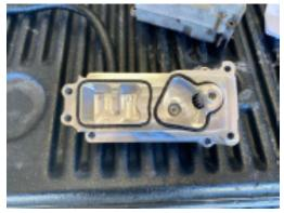
12.) Mount both halves together making sure to place the green gasket in between them in the proper orientation. Do not over tighten the retainers. Once they are tightened by hand evenly, it is now time to torque them. **TORQUE VALUE IS ONLY 25 IN-LBS.**
