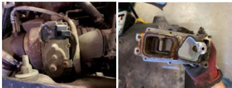
8.) Once the actuator is removed, clean the surface of where the old actuator was mounted.
