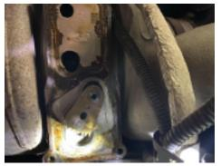
10.) Remove the 4 retainers that hold both actuator halves together. \*For 07.5-12 year models – you will need to separate the two halves and reuse the gear housing of the old actuator. Some of these may have tamper proof torx. For the 07.5-12 trucks, you need to make sure you get any water out of the gear housing before mounting the new actuator half to the old gear housing. If you get coolant in the actuator half for any reason you **WILL VOID** the warranty.
