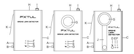
A-Power Socket; B- Smoke Outlet; C- Oil Level Gauge; D- Start/Stop Button; E- Power LED; F- Working Cycle LED; G- Pressure Gauge; H- Hook Port; I-Oil Refill Port; J- Flow Meter; K- Velcro Strap.
