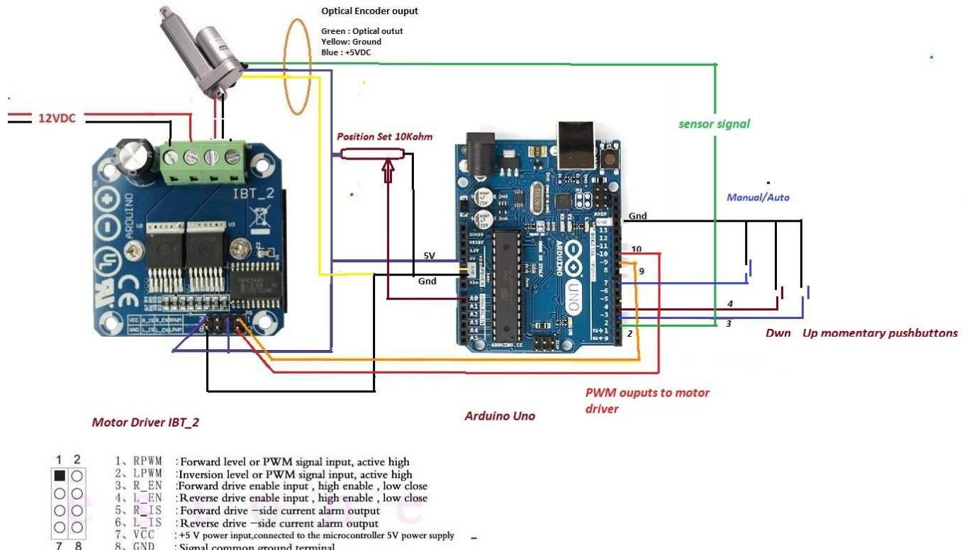
VCC pick MCU 5V power supply, GND connected microcontroller GND
