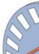
Let's say a disc has ten slots or holes in it and the disc is in the same location in the actuator as the magnetic disc in a Hall sensor setup. The resolution is now ten times more because there are now ten pulses per revolution instead of one. So, the 1000 pulses the Hall sensor would have read is now 10,000. The accuracy is calculated as  $10,000 / 24" = 416.66$  pulses per inch or 1 pulse per 0.0024" (0.06mm).
