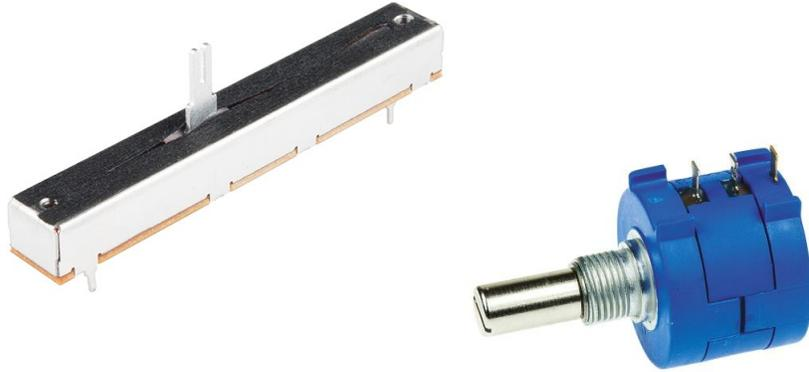
Above: Linear and Rotary Potentiometers
