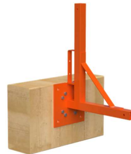
Parapet Installation with eight (8) 3/8" x 2-1/2" Lag Screw
