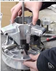
11. Using a T25 socket remove the stock flyweights. Remove the bolt and press the pin out of the clutch to remove the weight
