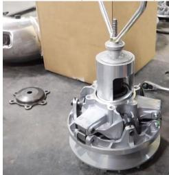
8. Compress the primary spring to expose the c-ring and remove the c-ring
