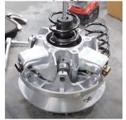
15. Reinstall the spring support and seat.
