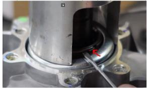
9. Decompress the clutch and then remove the stock primary spring.
