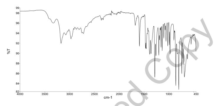
The interpretation of the signals of the Fourier-Transform Infrared Spectrum is consistent with the structural formula.
