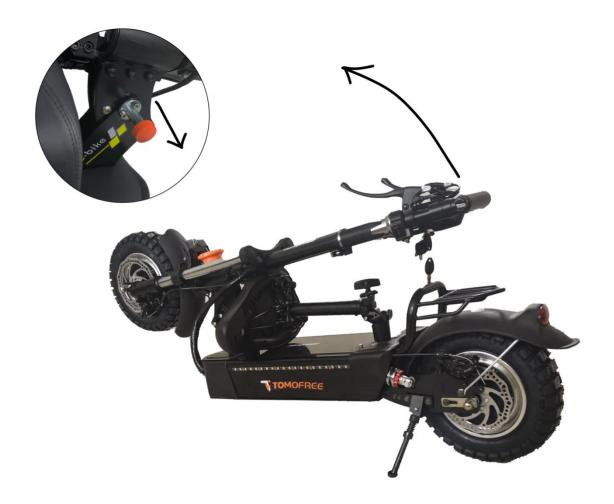
Step 3: Unfold the handlebar and rotate the turn buckle to hold it.
