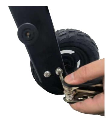
Step 3: Install the handlebar, tighten the two setscrews
