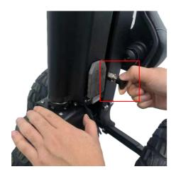
Step 2: Push up the buckle of the handlebar and unfold the handlebar
