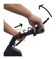
**Step:** Unfold the saddle
